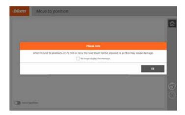
If you enter a dimension of 72 mm or less, a note will appear which says that the ruler could be damaged during knocking in. The rams are very wide. If the rulers are too close together during knocking in, the ram can damage the ruler.
