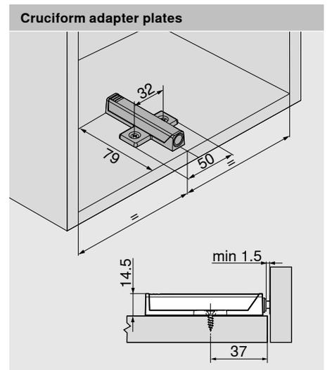
Installation dimensions for front gap
