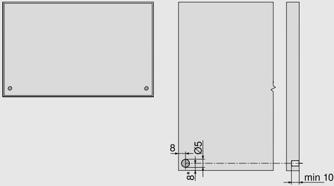
Recommendation for aluminium frames: Provide drill hole for the Blum distance bumper in the cabinet side. A trial application must be carried out when fixing the Blum distance bumper to the front.
