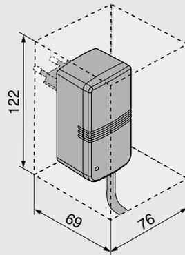
**i** A safety distance of 30 mm must be maintained for air circulation (see graphic); otherwise, there is a risk that the Blum transformer or plug-in transformer could overheat.
