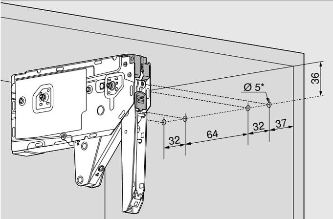
\* Drilling depth 11.5 mm
