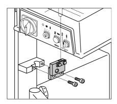
2. Changing control unit attachment (This only applies to machines with serial numbers up to AC100)
