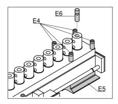
Loosen orange adjusting screws (E4) and then tighten slightly
